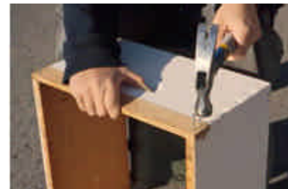
6. Nail it in but predrill the holes.
