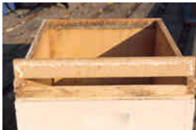
5. Cut out the damaged area and glue in the replacement parts.
